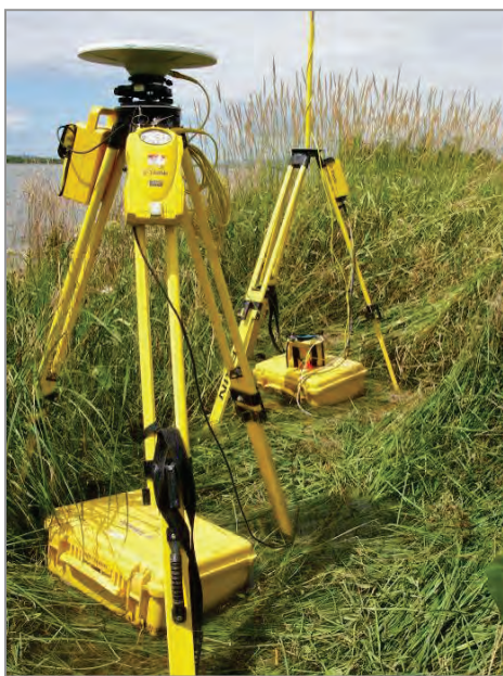
Figure 6. RTK base receiver set up near a study site to collect static data for the temporary benchmark used at the study site.
